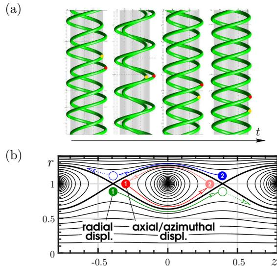
Fig. 3 (a) Elementary event in the nonlinear dynamics of two helical vortices. (b) Iso-Hamiltonian lines in the  $(r, z)$  plane, showing several types of vortex trajectories.
