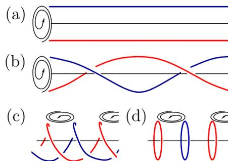
Fig. 1 Merging of vortices: (a) straight vortices, (b) large-pitch helical vortices, (c) small-pitch helical vortices, (d) array of vortex rings. The arrows qualitatively indicate the merging dynamics.
