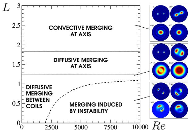
Fig. 2 Merging of two helical vortices: different scenarios in the  $(Re, L)$  plane. Right: typical time evolutions of  $\omega_B$  in a plane orthogonal to the helix axis.
