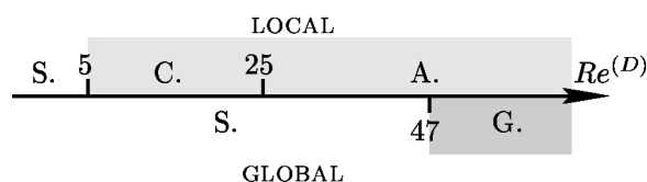
FIG. 1. Local versus global instability properties of the two-dimensional cylinder wake. S: stable, C: existence of a convective instability pocket, A: existence of an absolute instability pocket, G: globally unstable. Grey areas denote instability.
